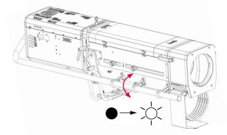
Step 4 - The light beam zoom and focus can be set by using the control knobs A & B
